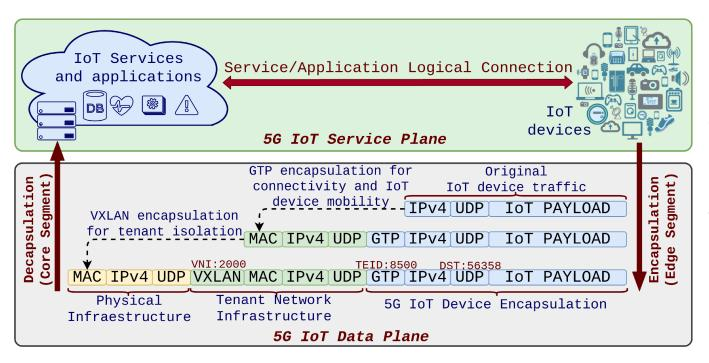
The same original IoT packet transmitted by an IoT device or sensor can have different packet structure with different encapsulation and tunnelling headers depending on the network segment.
